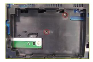
6. Disassemble ODD from system. Pull ODD to left.
