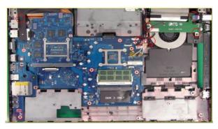
10. Remove 2 Cables, DC Cable & LCD Cable
