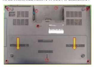
**4.** Open the HDD door to disassemble. And remove 12 Screw & HDD protect cover.
