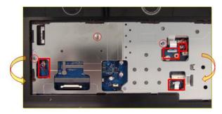
**9.** Remove 7 screw to disassemble.
