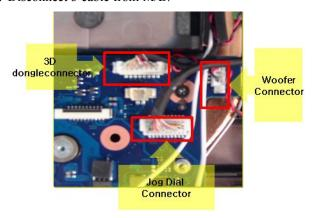
**13.** After disconnect, you can seprate M/B from Bottom ASSY. And Disconnet Fan Cable and Heat Sin.
