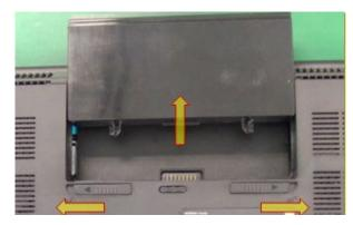
**2.** Remove the dummy-SD CARD before disassembling.
