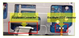
8. Remove 3 screws, at ○ point. Disconnect 2 FFC Cable & 2 speaker Cable, at □ Point. After this, open the top assy from bottom.
