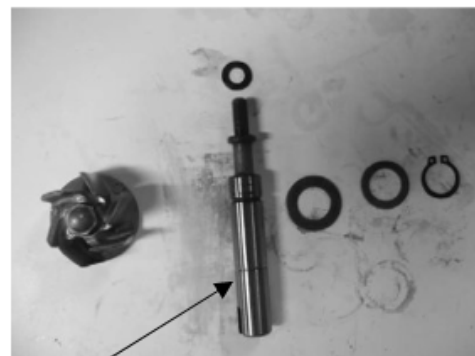
Water pump shaft
